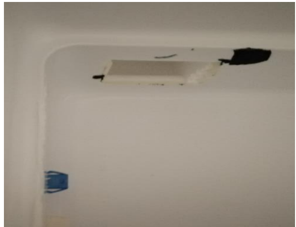
Freezer → air supply outlet of fridge
