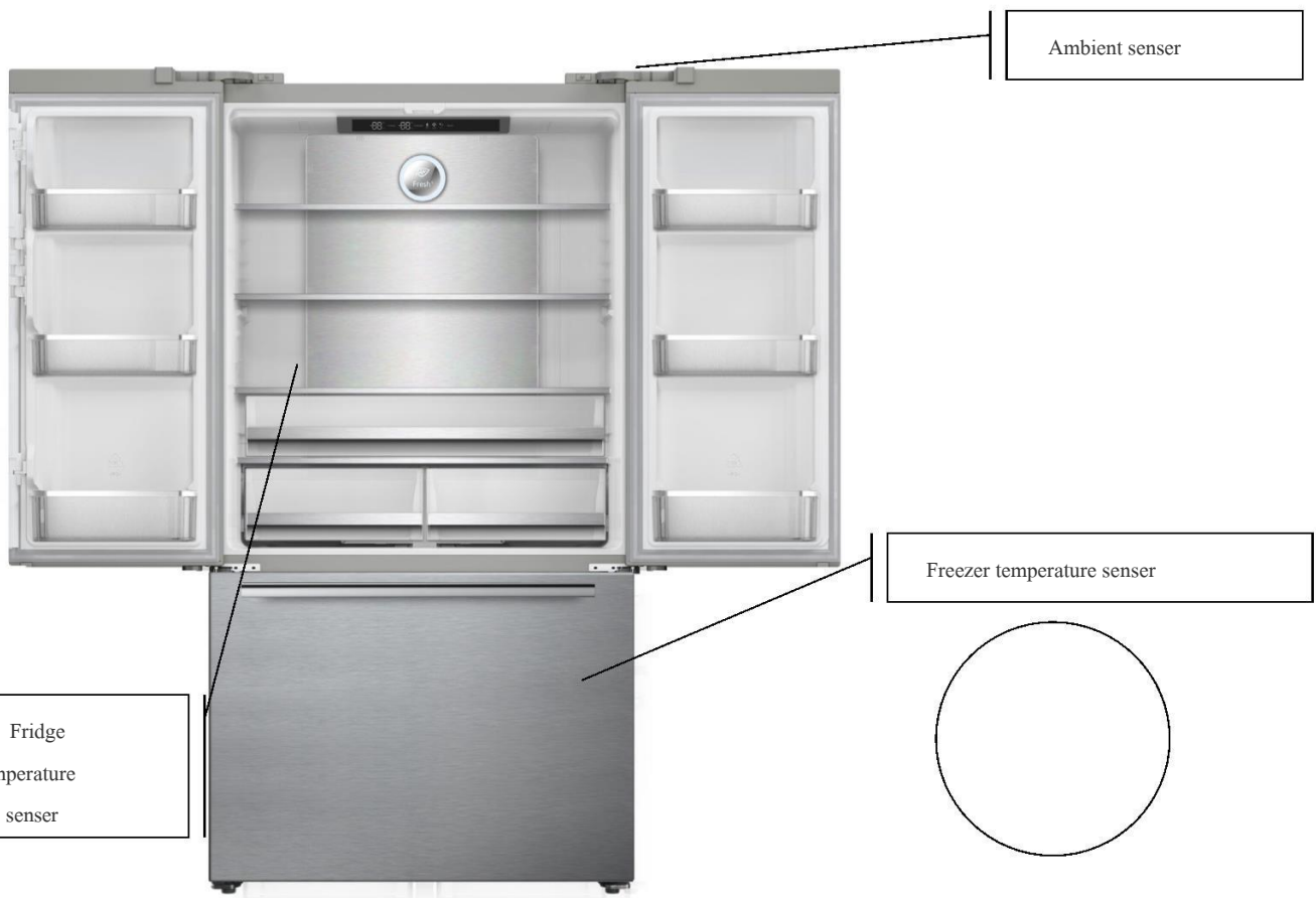
Freezer sensor and fridge sensor location
